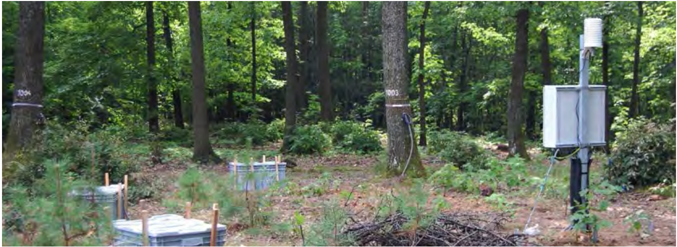
Weather station, stem growth measurements and boxes for soil solution measurement equipment, Austria.
