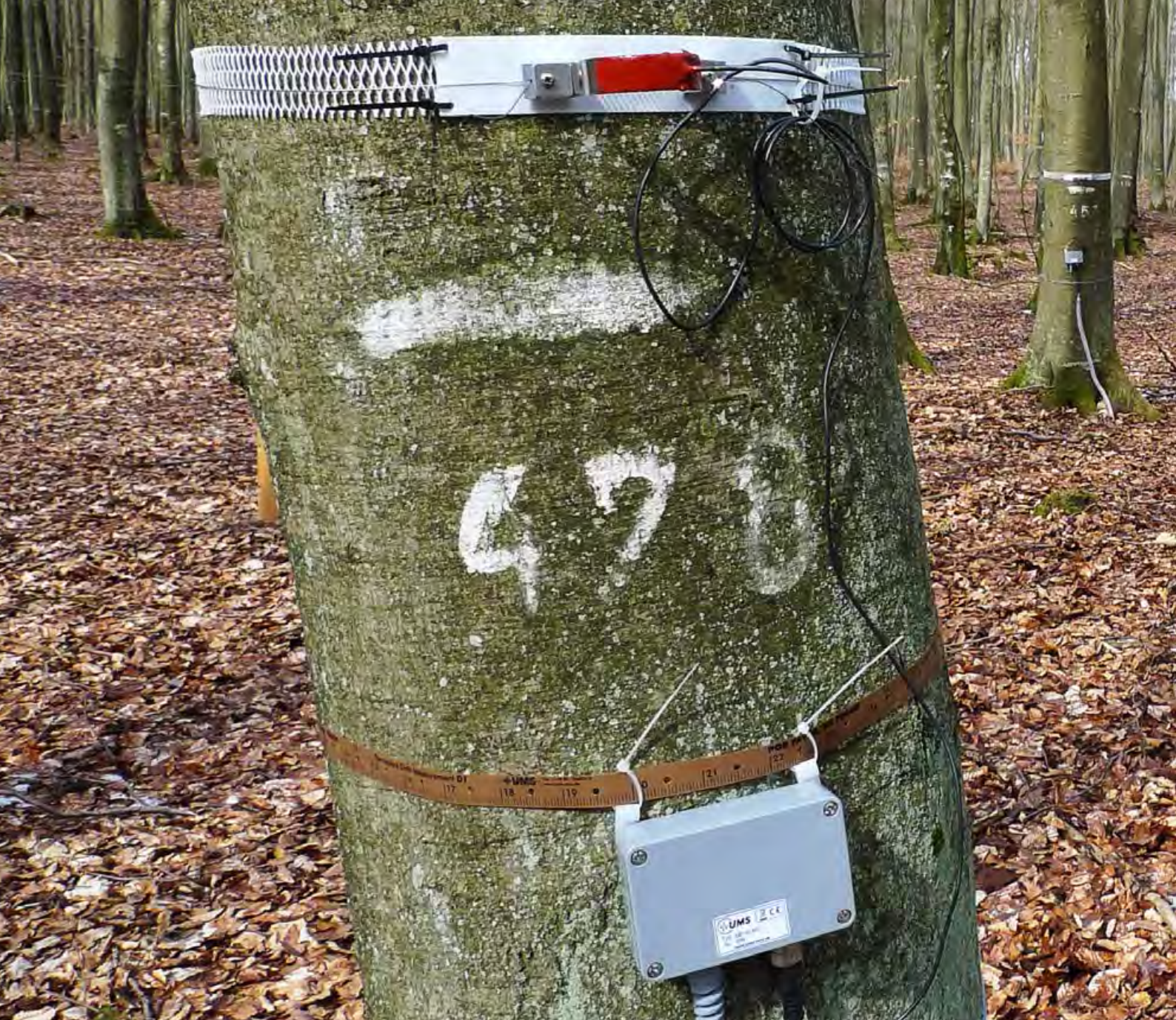
Continuous stem growth measurements on a Level II plot, as well as deposition measurement equipment for stemflow (black bin) and throughfall (orange samplers), Poland.
